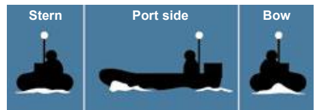
A standard power-driven vessel – less than 7m in length, less than 7 knots speed, should display an all round white light. (As a bare minimum)
