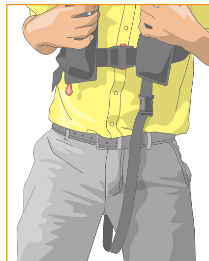
Crotch strap too loose
